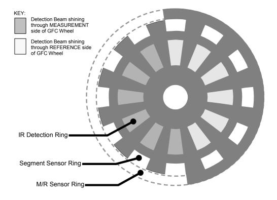
Figure 13-11: GFC Light Mask
